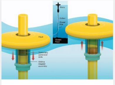
the sliding magnet assembly coupled to the float. (Image courtesy of Smithsonian Magazine) E. Rusch, \*Catching a wave, powering an electrical grid?, \* Smithsonian Magazine, July 2009.
